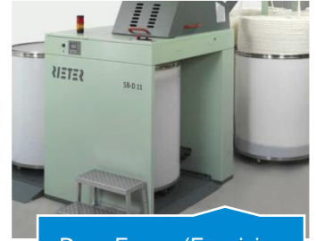
Draw Frame (Evenising and Parallelizing of fibre)
