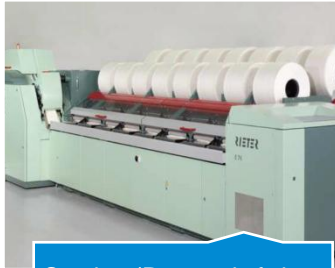
Comber (Removal of short fibre)
