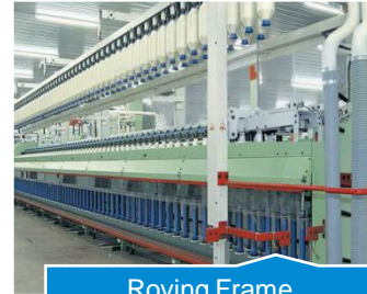
Roving Frame (Intermediate stage of Yarn forming)
