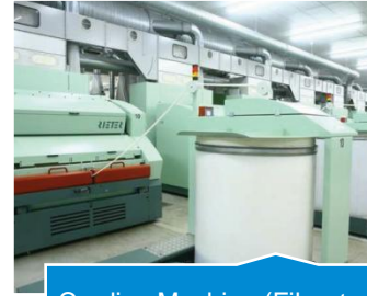
Carding Machine (Fibre to Fibre preparation)
