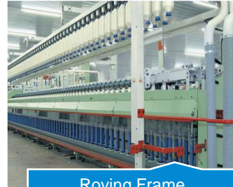
Roving Frame (Intermediate stage of Yarn forming)
