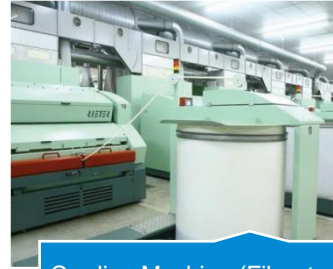
Carding Machine (Fibre to Fibre preparation)
